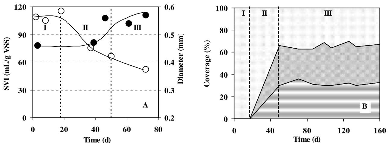
**Figure 4.** A) Sludge volumetric index (SVI) (○) and average feret diameter (●). B) Percentages of zeolite fully covered (▤), partially covered (▨) and no covered (□).
