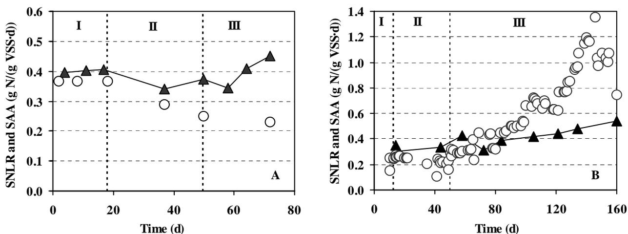
**Figure 1.** Specific Nitrogen Loading Rate (SNLR) applied (○) and Specific Anammox Activity of the biomass (SAA) (▲) in reactors SBR1 A) and SBRZ B).
