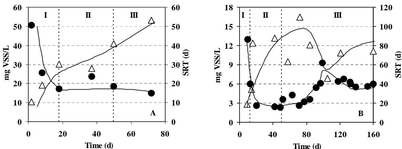
**Figure 3.** Biomass concentration in the effluent (mg VSS/L) (●) and sludge retention time (SRT, d) (Δ) in reactors SBR1 A) and SBRZ B).
